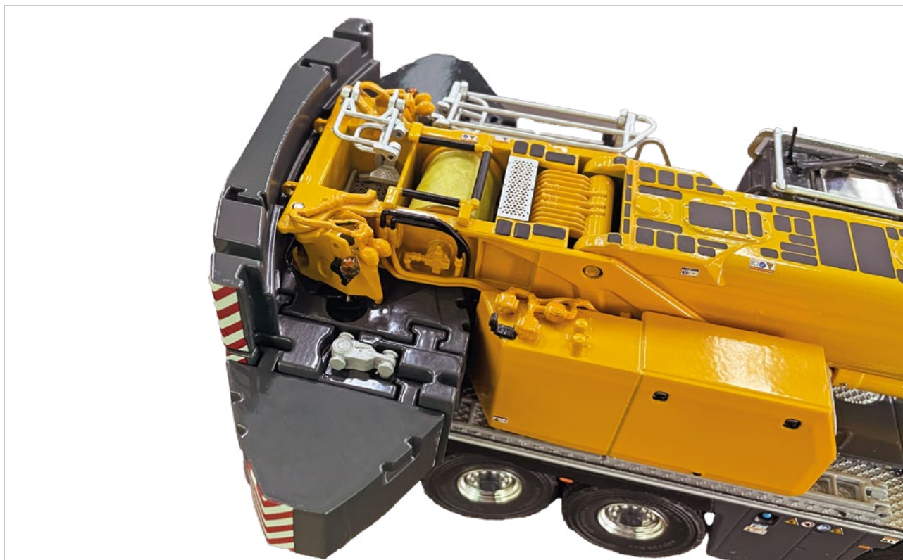
Ballast package front position. The position can be changed by loosening the two bolts in the next step.
