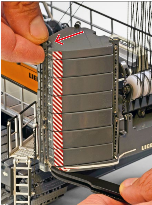
Connect the lashing at the top of the ballast blocks
