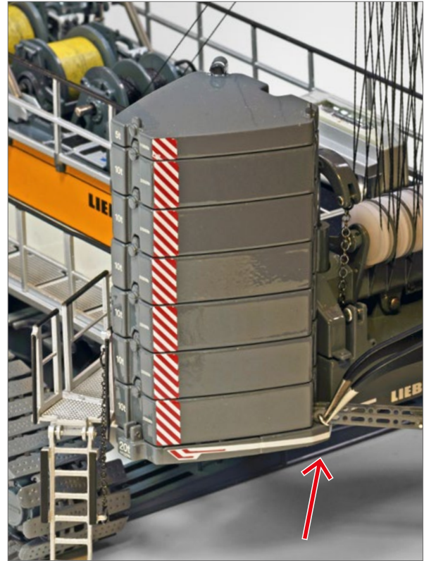
Connect the lashing at the bottom with the bended pin (B9Z)
