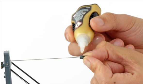
Knot and glue the end of the rope to the rope lock part (B9F)
