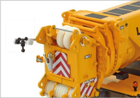
Anemometer (windspeed indicator).
