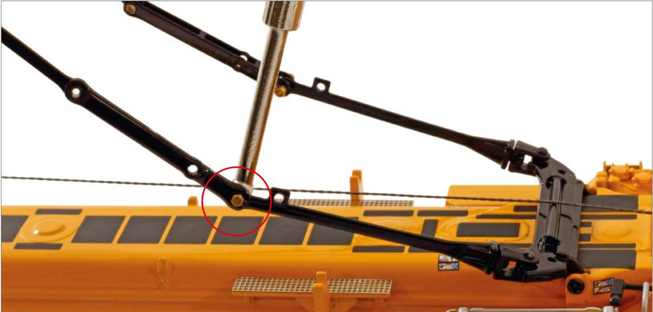
Secure TY rods to parts #16 by using nut/bolt #39 and tool #26 and #27.
