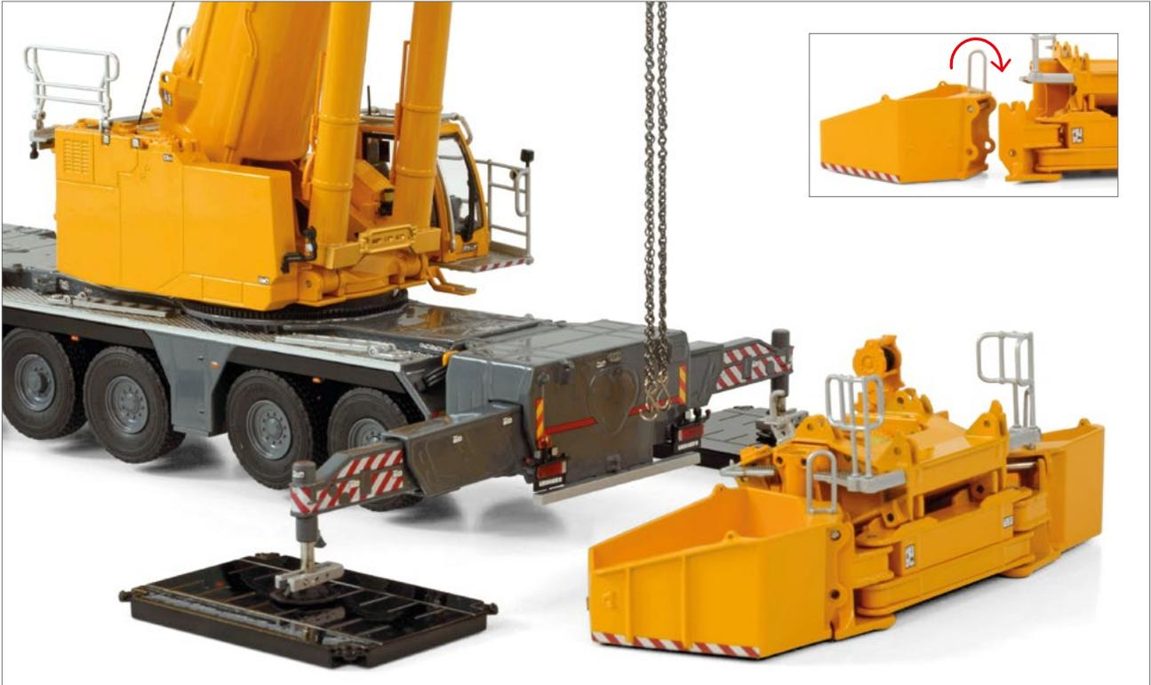
Add receptacle plate to counterweight frame and secure it using pin #32.
