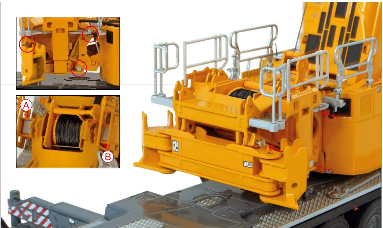
Secure the counterweight baseplate at three points by using pins #33, #35 and #39. Install counterweight baseplate covers at indicated points (A and B).
