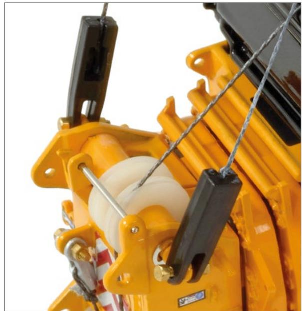
Connect the loose ropes to boom head by using bolts and nuts #38 and tool #26 and #27.
