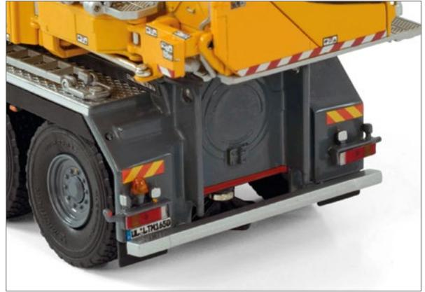
Rear bumper. Always remove before outrigger box installation.
