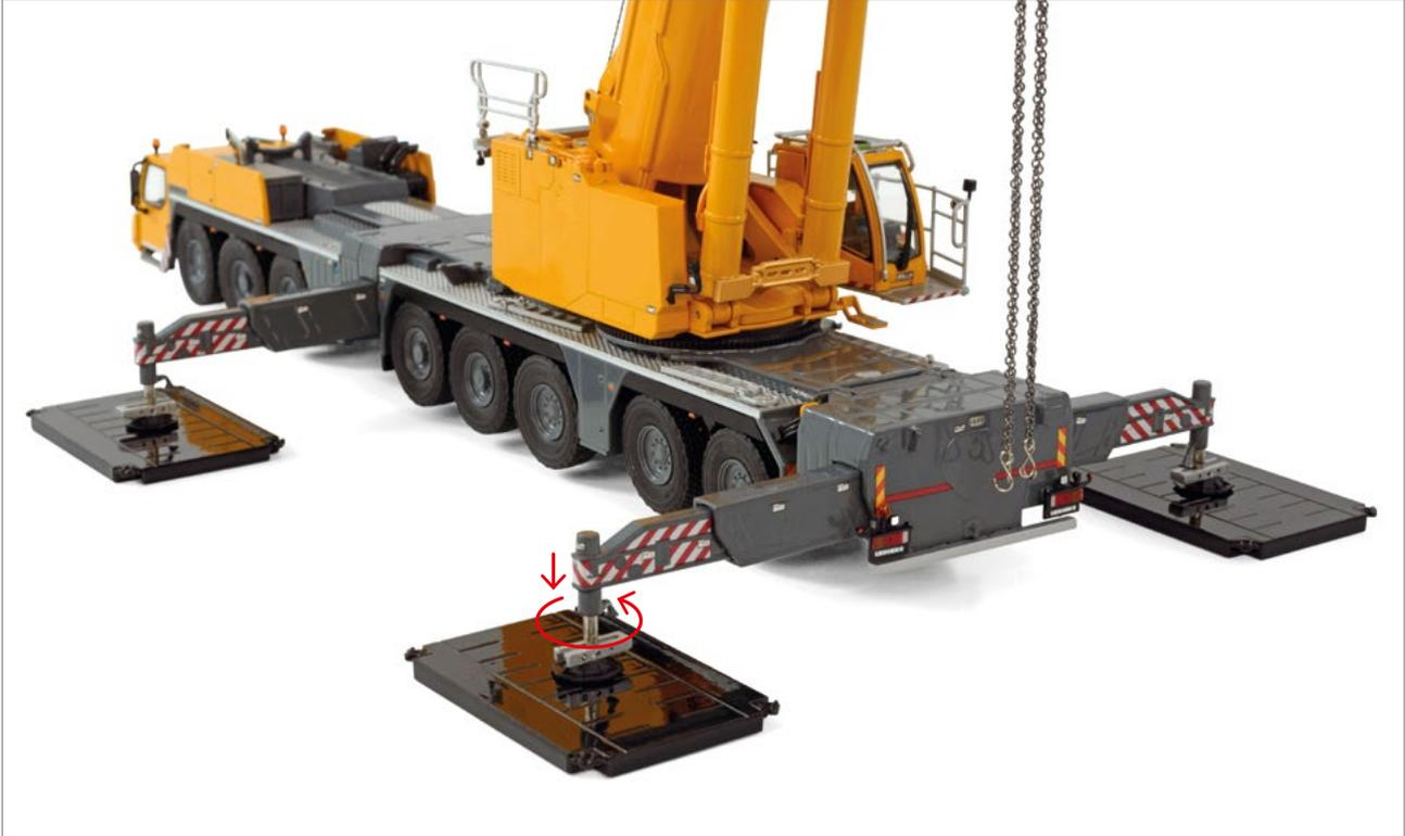
Overview photo. Make sure the crane is level and in stable position.
