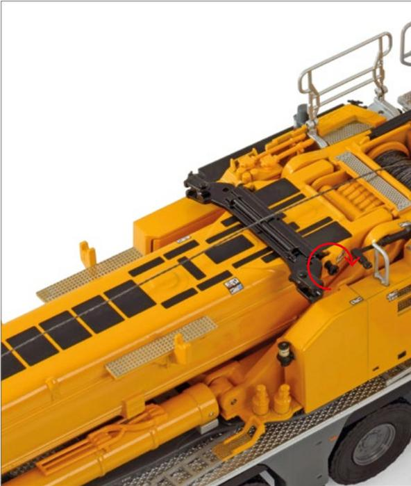
Install the rod connector to the main boom. Use screw #41 and a screwdriver to secure the rod connector.
