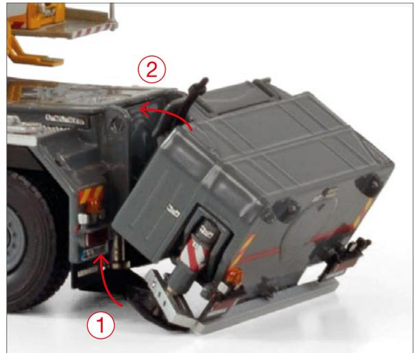
Attach outrigger box to back of the crane.
