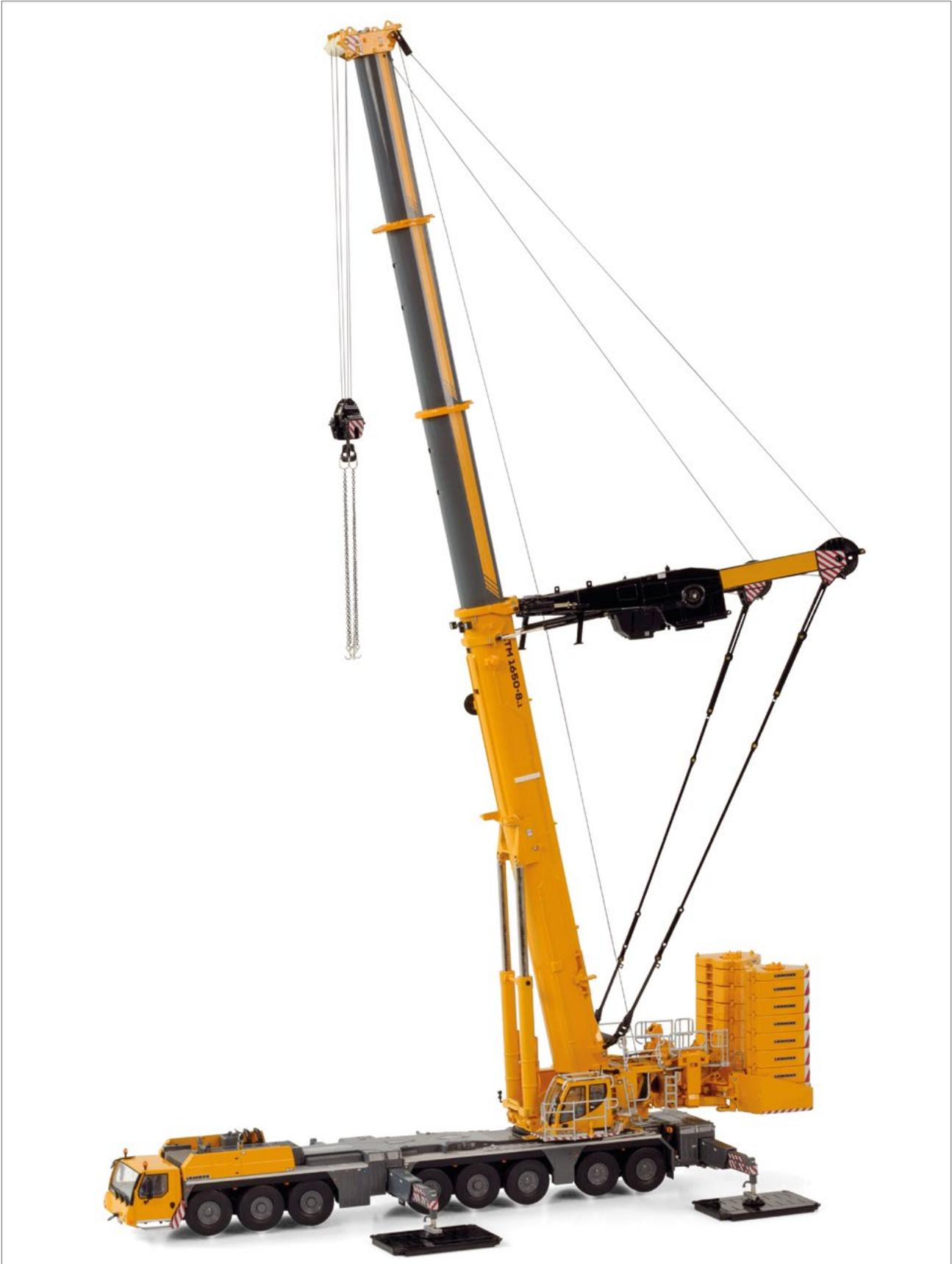
TY3 configuration. To tension up the TY-Guying system, carefully wind up the TY winches using tool #28.
