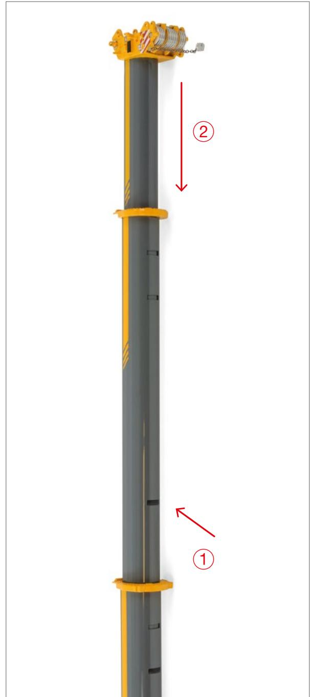
Simultaneously push the smallest boom section downwards into the next bigger section until it is completely retracted. Repeat these steps for the remaining boom sections.
