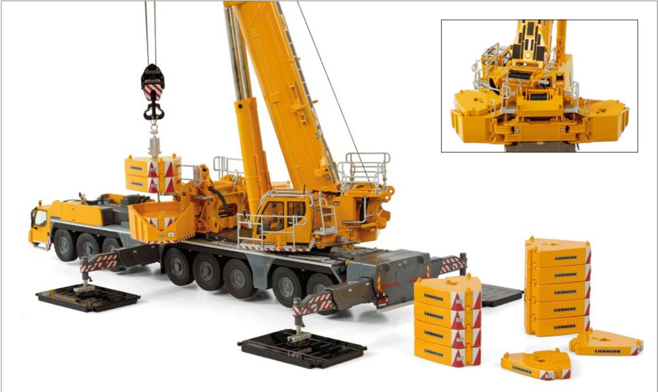
Place two blocks at the right side, then two blocks at the left side. Counterweights can be stacked with max 10t difference per side.
