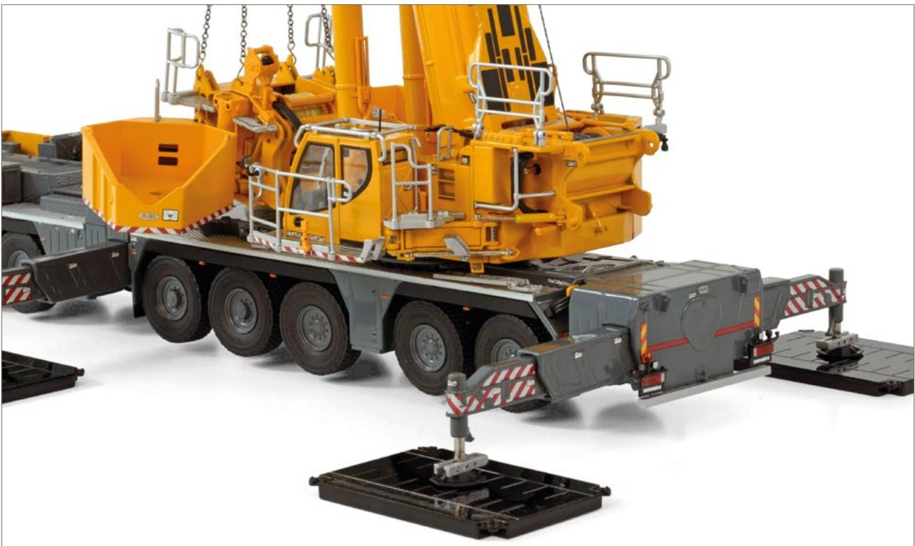
Lift counterweight assembly onto the undercarriage using the lifting chains (#47).
