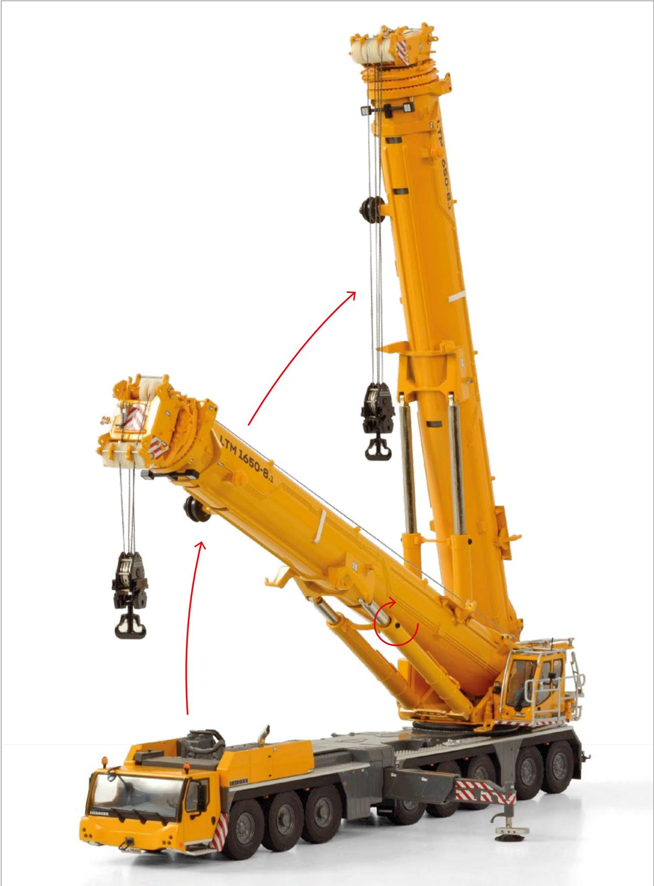
Luff the boom and secure the hexagon bolt using tool #29.
