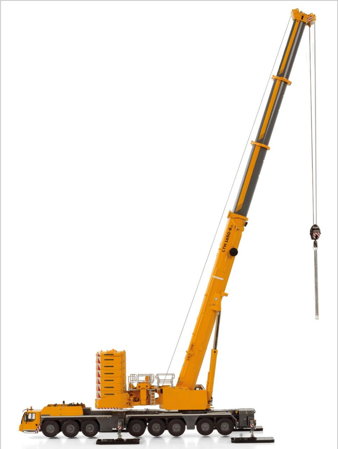
T3 configuration, boom at 46% position. It is also possible to extend to 92% and 100%.
