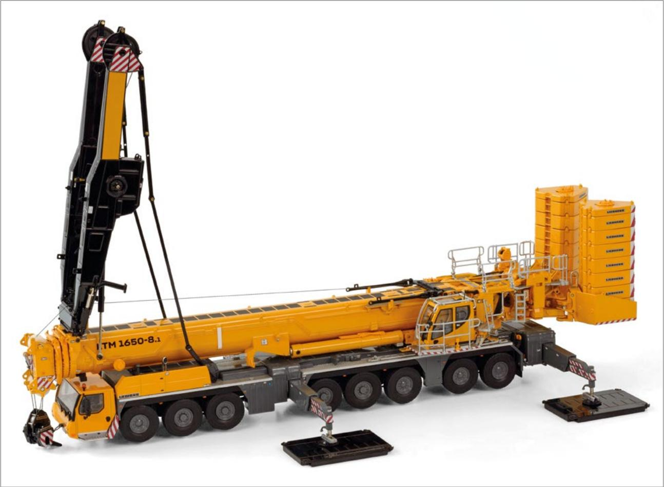
TY arms in upward position prior to installation of rods.
