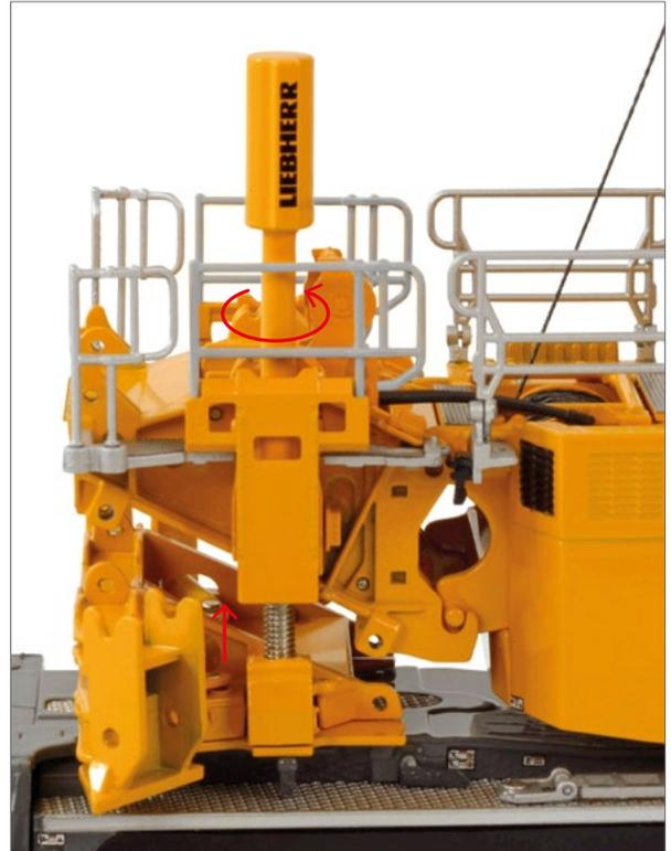
Use tool #28 to raise the counterweight baseplate until it lines up with the connecting points of the uppercarriage. (On the photo the counterweights are left away to get a better view of the process).
