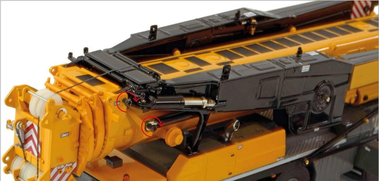
Secure TY-Guying system using screw #40 by screwdriver, then secure TY-Guying system cylinders using screw #41 by screwdriver.
